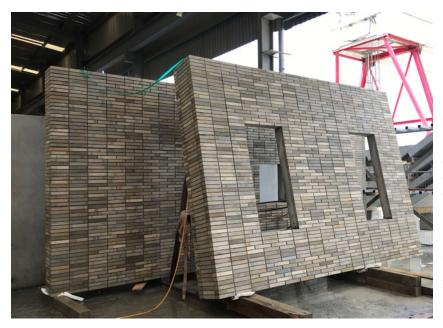
Because behind this unique facade was a rigorous process involving checking Brick Inlay's performance in key earthquakes zones of Los Angeles and San Francisco (a strong tick), six months of thorough compliance testing using mock-up panels, and refining the design and construction based on those results.
